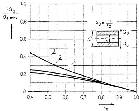
Fig. 6. Axial stress maxima at the outer side
