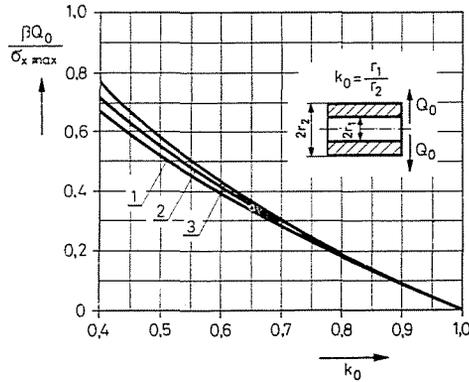
Fig. 5. Axial stress maxima at the inner side
