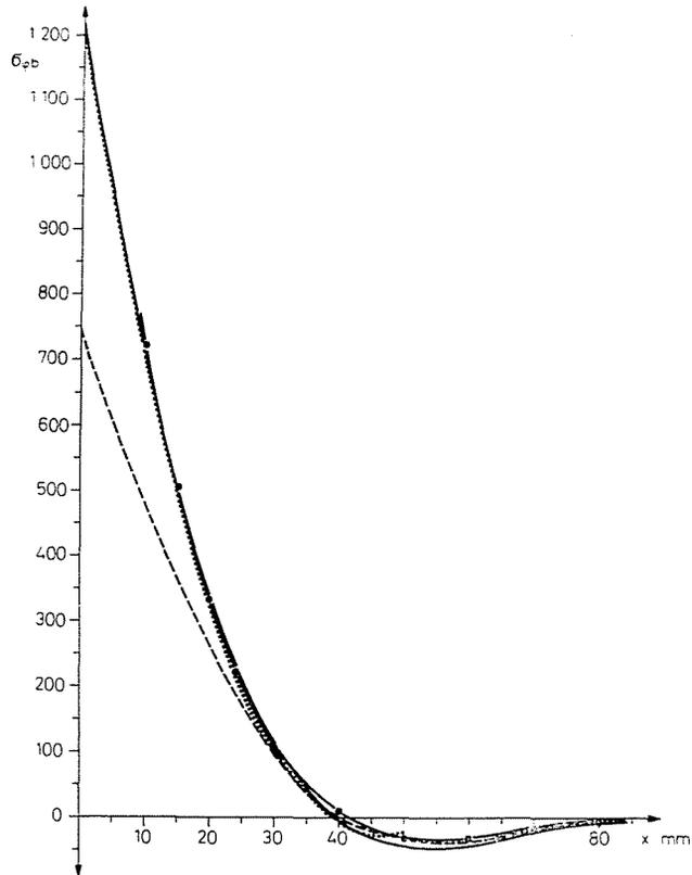
Fig. 10. Tangential stress due to load  $P = 4000$  kp at the inner tube side. According to the modified method: full line; according to the shell theory: dashed line; according to the Biederman method: dotted line; measured: discrete points
