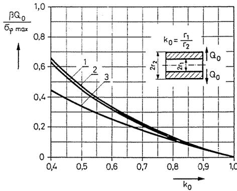
Fig. 8. Tangential stress maxima at the outer side
