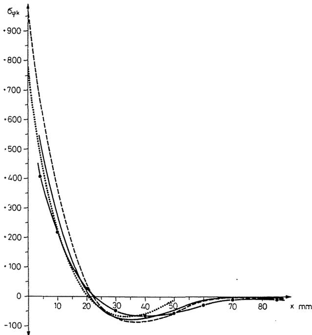
Fig. 11. Tangential stress due to load  $P = 4000$  kp at the outer tube side. According to the modified method: full line; according to the shell theory: dashed line; according to the Biederman method dotted line; measured: discret points
