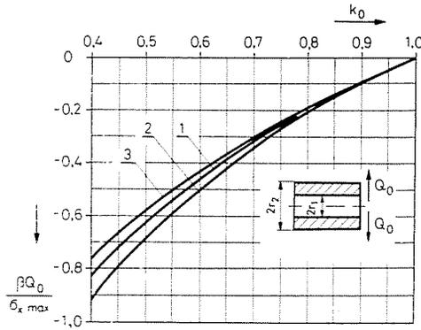
Fig. 7. Tangential stress maxima at the inner side
