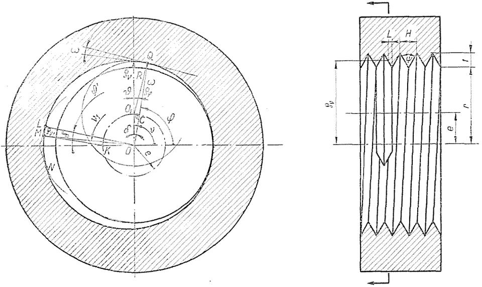
Fig. 6. Relative positions of the tool and the workpiece
