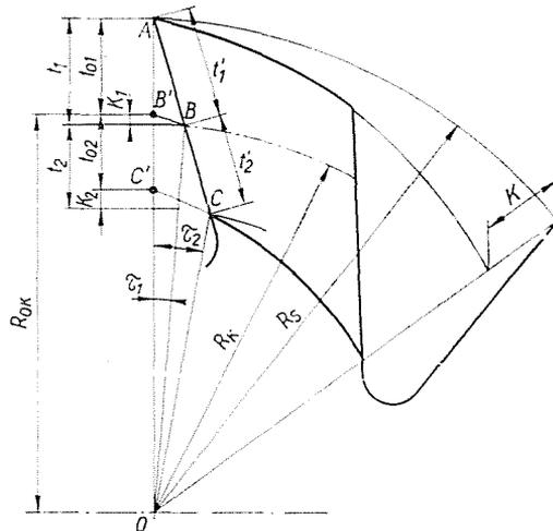
Fig. 8. Analysis of the profile elements of the tool with positive rake angle
