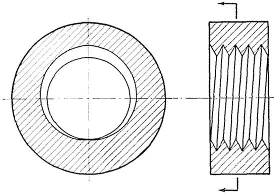
Fig. 4. Cross-section of the workpiece
