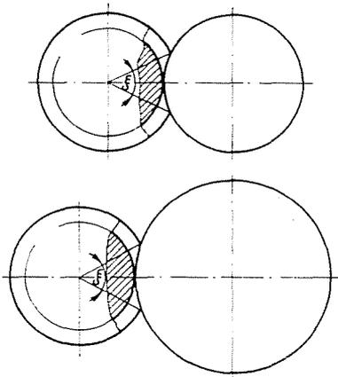
Fig. 1. Length of engaging arc between tool and workpiece in external thread cutting
