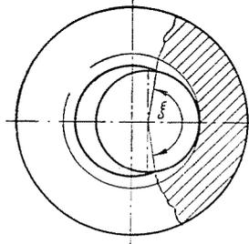
Fig. 2. Length of engaging arc in internal thread cutting
