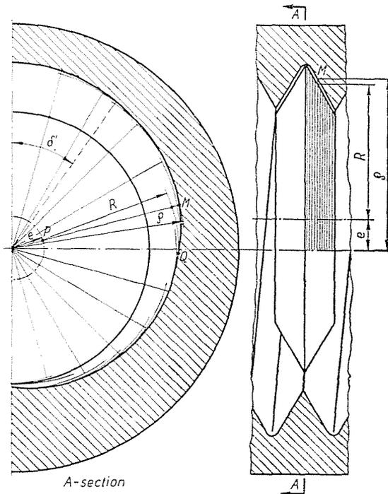
Fig. 5. Construction of helix in the section normal to the axis, in internal thread cutting
