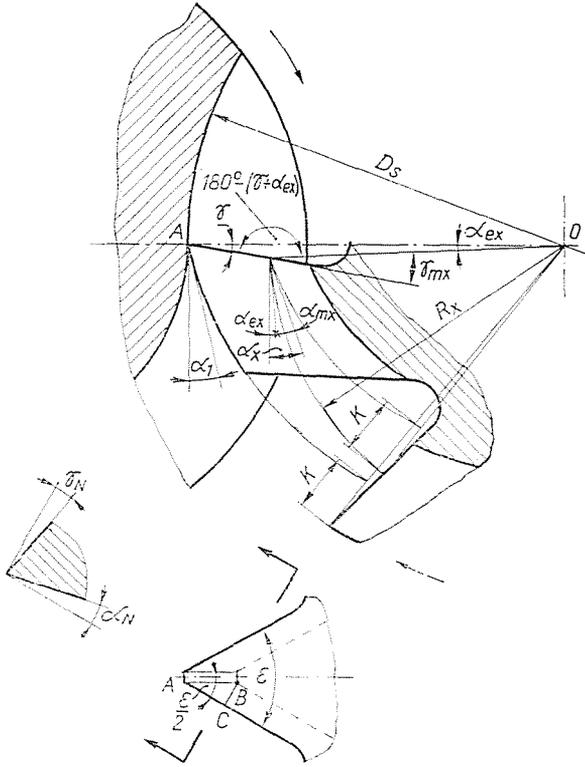
Fig. 3. Position of the thread milling hob and the workpiece during the machining process
