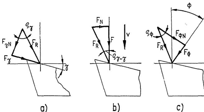
Fig. 2. Components of cutting force
