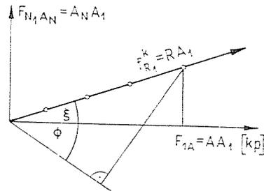
Fig. 8. Calculation of mean shear stress
