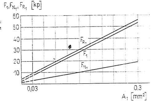
Fig. 4. Scalar values of main cutting force and its components
