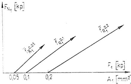
Fig. 5. Vectors of cutting force
