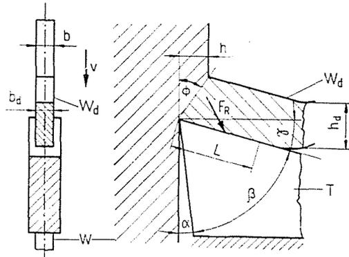
Fig. 1. Elements of cutting process
