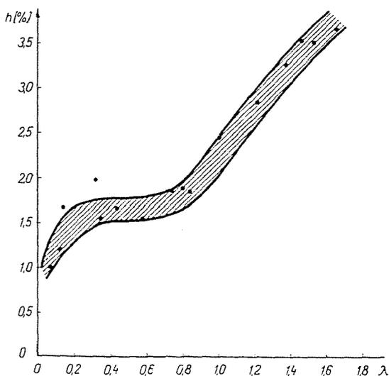
Fig. 5. Error in temperature gauging vs. true strain
