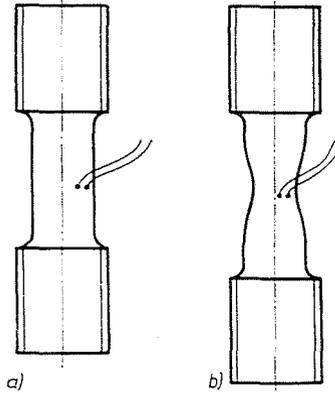
Fig. 4. Shape of the tensile specimen up to the limit of uniform true strain (a) and following the beginning of contraction (b)
