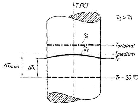
Fig. 2. Schematic diagram for notating temperature variations in the tensile specimen
