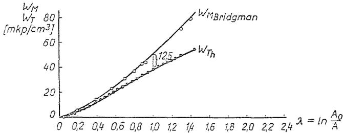
Fig. 4. The curves for tensile stress according to the mechanical work assumed by Bridgman and of the energy transformed into heat while drawing were plotted
