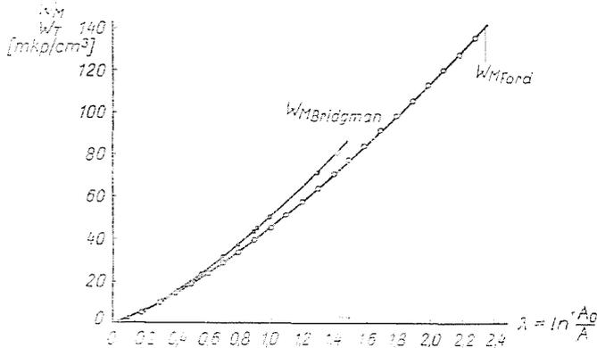
Fig. 2. The changes in mechanical work as a function of strain
