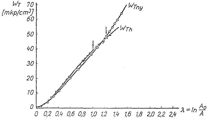
Fig. 3. The part of external work transformed into heat
