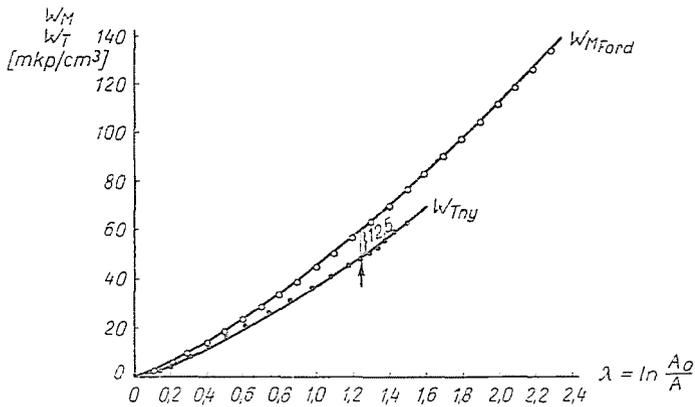
Fig. 5. The curves for mechanical work in case of compressive stress and for the energy released while compressions were plotted
