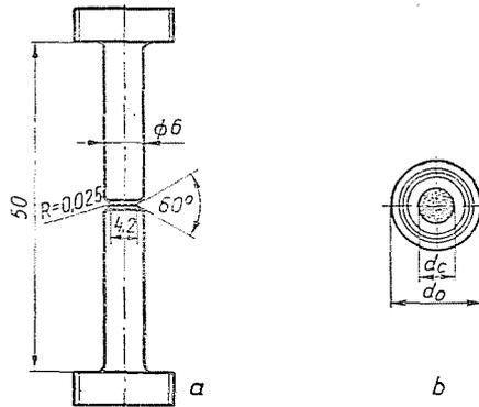
Fig. 8. a) Tensile stress test specimen, b) Fractured test specimen cross section
