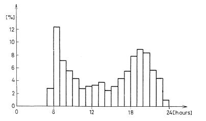
Fig. 4a. Pattern of the hot tap water consumption of a 32-flat block - on weekdays
