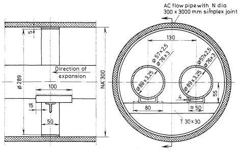
Fig. 8. Laying of transmission pipes with asbestos cement pipes
