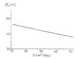
Fig. 5. Correlation of the temperature and quantity of hot tap water
