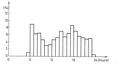
Fig. 4c. Pattern of the hot tap water consumption of a 32-flat block - on Saturdays
