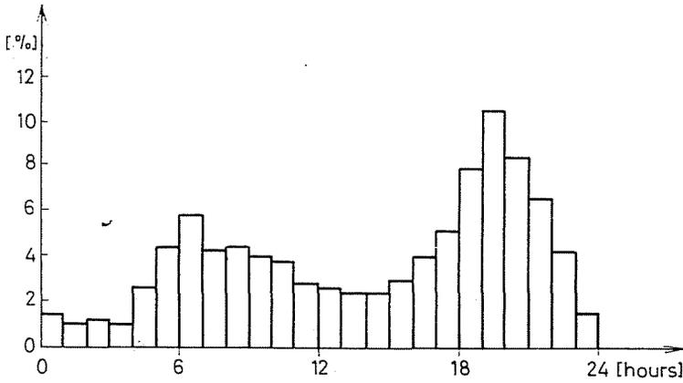
Fig. 4b. Pattern of the hot tap water consumption of a 100-flat block — on weekdays
