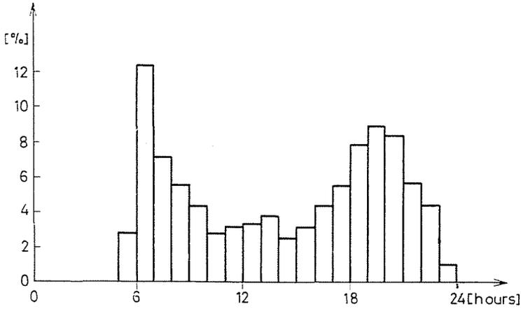
Fig. 4a. Pattern of the hot tap water consumption of a 32-flat block — on weekdays
