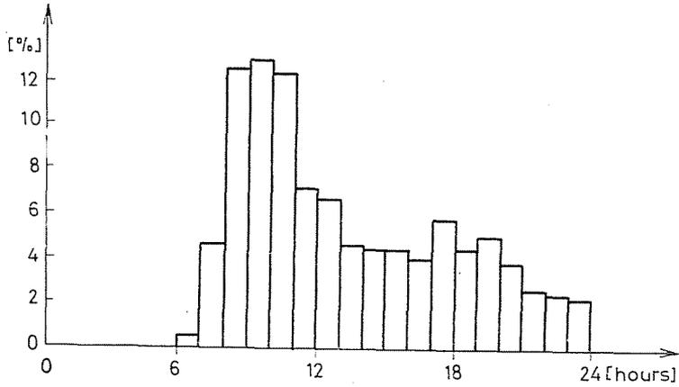
Fig. 4e. Pattern of the hot tap water consumption of a 32-flat block — on Sundays
