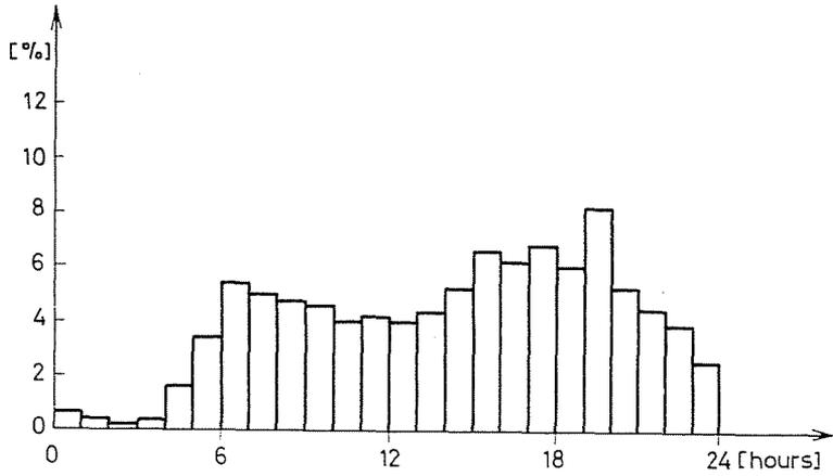
Fig. 4d. Pattern of the hot tap water consumption of a 100-flat block — on Saturdays
