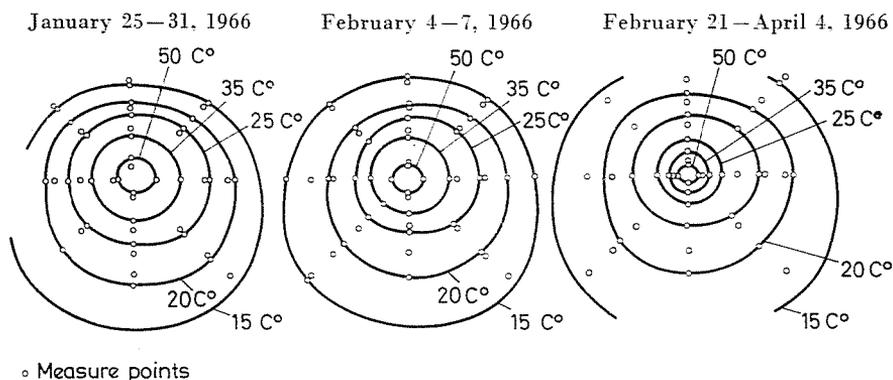
Fig. 9. Isotherms dia. 300 asbestos cement pipe without insulation
