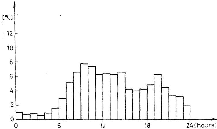
Fig. 4f. Pattern of the hot tap water consumption of a 100-flat block — on Sundays
