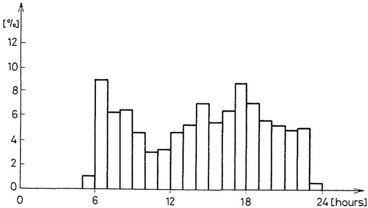
Fig. 4c. Pattern of the hot tap water consumption of a 32-flat block — on Saturdays
