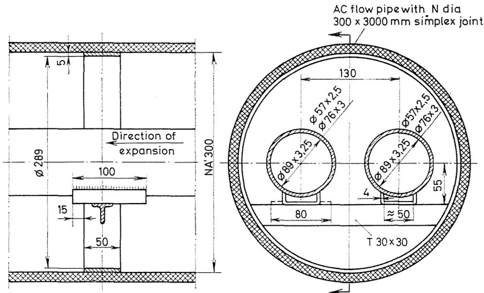
Fig. 8. Laying of transmission pipes with asbestos cement pipes
