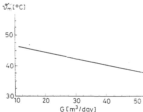
Fig. 5. Correlation of the temperature and quantity of hot tap water
