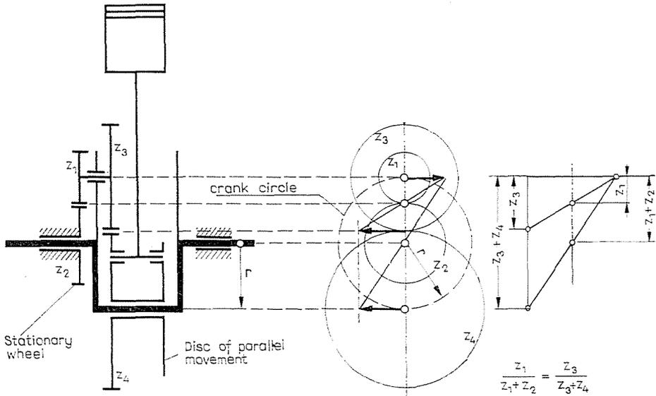
Fig. 1. Nordberg two-stroke cycle 11 cylinder radial engine.  $N_e = 1700$  HP;  $n = 400$ /min.;  $V_H = 400$  lit.;  $S/D = 406/355$  mm
