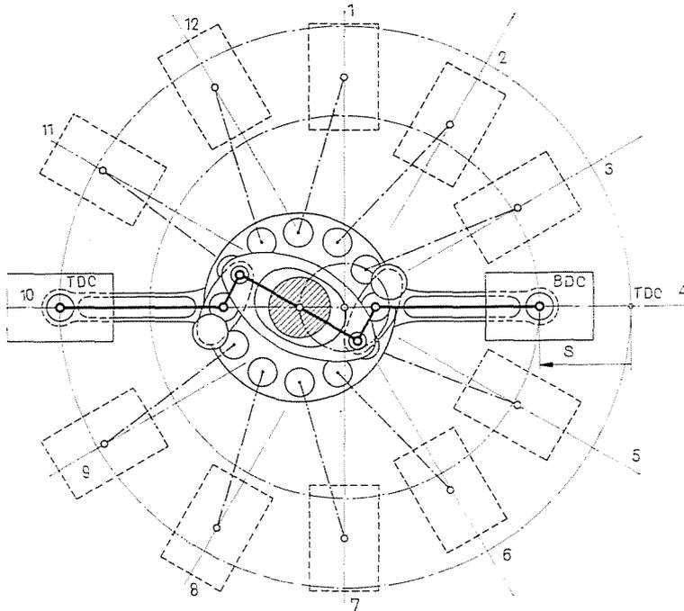
Fig. 2. Crank gear of the Nordberg two-stroke cycle 12 cylinder radial engine
