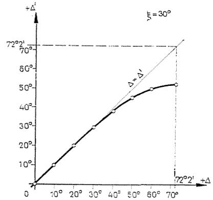
Fig. 9. Displacement of moving arms ( $\xi = 30^\circ$ )
