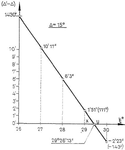
Fig. 12. Finding out the equal displacement position of the two moving arms
