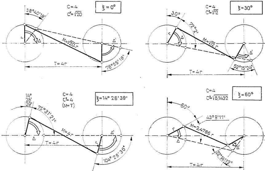
Fig. 6/a. Extreme positions of the mechanism with the starting position  $\xi = 0^\circ$
