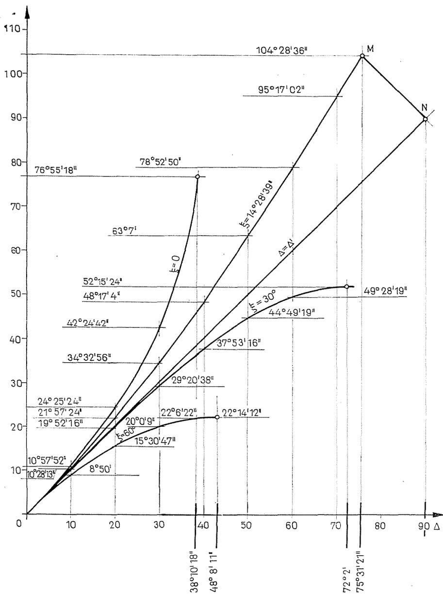
Fig. 11. Representation of displacement conditions of antiparallelogram mechanism fitted with moving arms, of different basic positions, in a combined diagram
