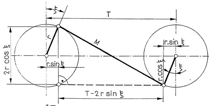
Fig. 5. Dimensions of the antiparallelogram mechanism
