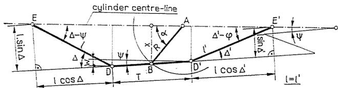
Fig. 14. Showing the position of the central disc represented by  $D-D_3$  in a general position of the crank mechanism (for finding out the displacement angle  $\psi$ )
