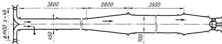
Fig. 6. Schlünkes' test setup with radial cascade
