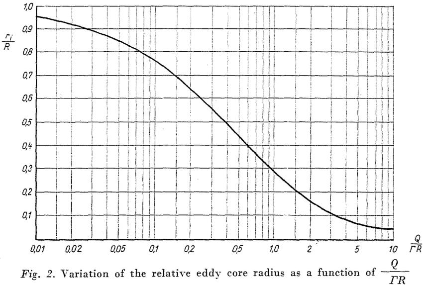
Fig. 2. Variation of the relative eddy core radius as a function of  $\frac{Q}{\Gamma R}$
