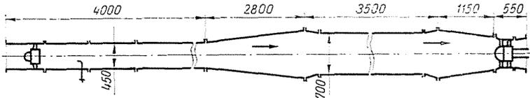
Fig. 7. Schlünkes' test setup with axial cascade
