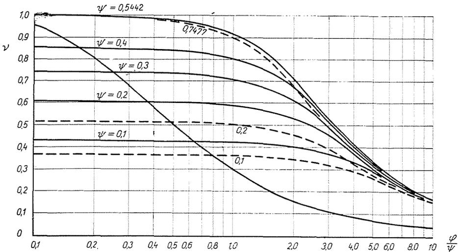
Fig. 16. Chart for the determination of the relative hub dimensions
