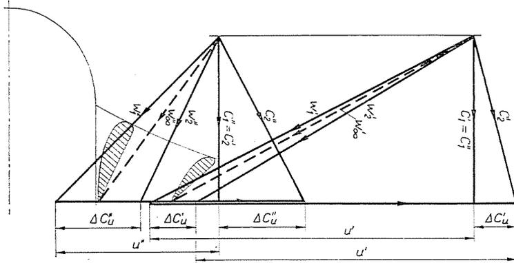
Fig. 13. Variation of the velocity triangles along the blade
