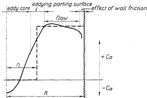
Fig. 3. Distribution of axial velocity with friction
