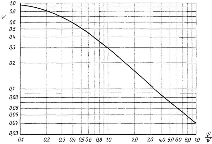
Fig. 15. Curve defining prevention of eddy core from forming
