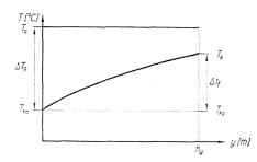
Fig. 2. Average temperatures of the medium and the fin base in the function of distance from the inlet
