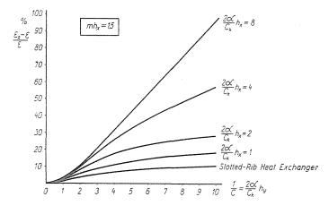
Fig. 3. Error due to neglection of the heat conductance in flow direction and the nonuniform changes in the temperature of the medium (at  $mh_x = 1.5$ )
