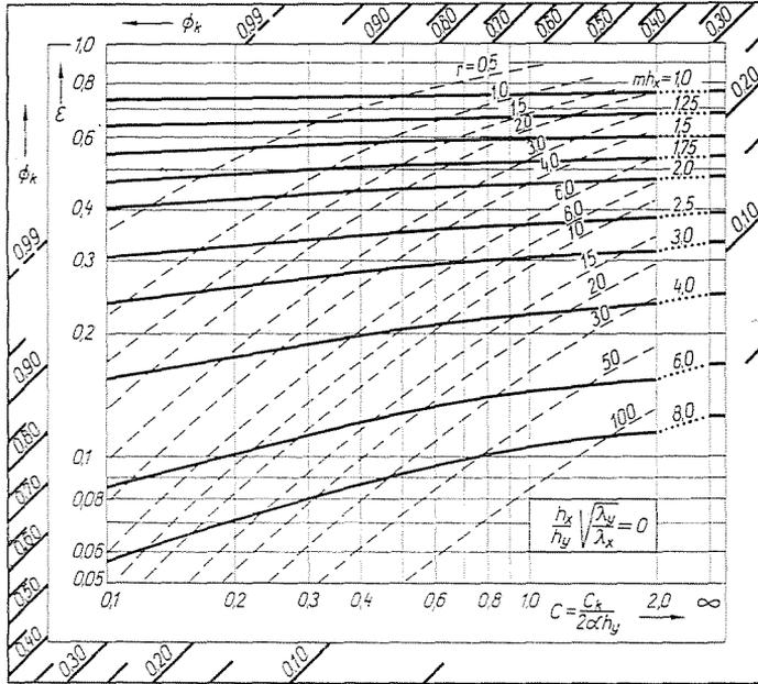
Chart 1. Accurate plate fin efficiency which takes into consideration the heat conductance of the fin in flow direction and the non-uniform changes in the temperature of the flow medium
