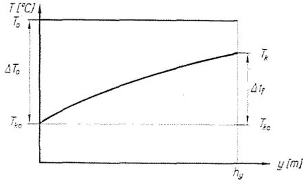
Fig. 2. Average temperatures of the medium and the fin base in the function of distance from the inlet
