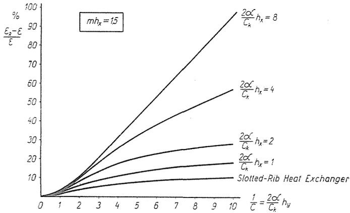
Fig. 3. Error due to neglect of the heat conductance in flow direction and the non-uniform changes in the temperature of the medium (at  $mh_x = 1.5$ )
