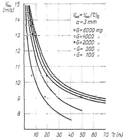
Fig. 5. Relationship between flow velocity and time of erosion test ( $\tau$ ), with constant eroded volumes ( $G$ ):  $v_{\infty} = v_{\infty}(\tau)_G$
