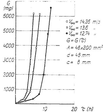
Fig. 4. Eroded volume ( $G$ ) in the function of time of the erosion test ( $\tau$ ), with different flow velocities ( $v_\infty$ ). Thickness of lead plate:  $a = 8$  mm
