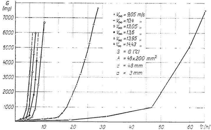
Fig. 3. Eroded volume ( $G$ ) in the function of time ( $\tau$ ) of the erosion test, with different flow velocities ( $v_\infty$ ). Thickness of lead plate:  $a = 3$  mm
