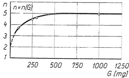
Fig. 7. Velocity-damage exponent ( $n$ ) in the function of eroded volume ( $G$ )
