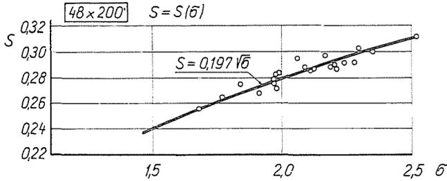
Fig. 8. Strouhal number ( $S$ ) in the function of cavitation number ( $\sigma$ )
