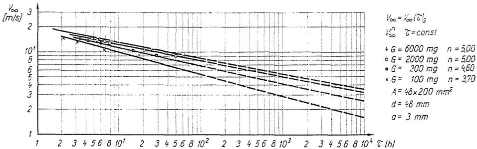
Fig. 6. Relationship between flow velocity ( $v_{\infty}$ ) and the time of erosion test ( $\tau$ ), with constant eroded volume ( $G$ ),  $\lg v_{\infty} = \lg v_{\infty}(\lg \tau)_G$
