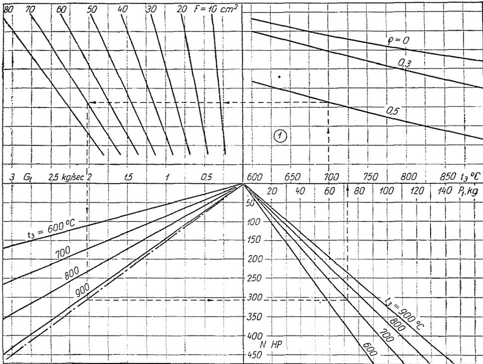
Fig. 4. Diagram for determining the output and thrust of gas turbines
