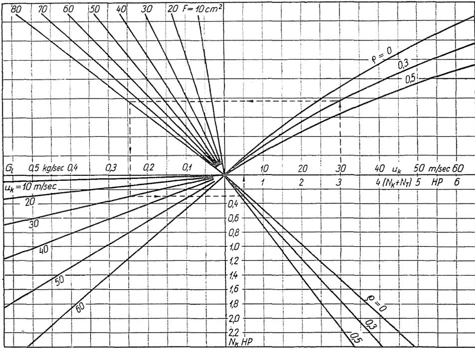
Fig. 6. Alteration of the starting of power requirement of a "cold" gas turbine
