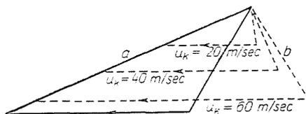
Fig. 5. Modification of the turbine speed triangles in case of cold and warm condition resp. a) warm condition, b) cold condition
