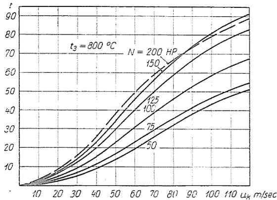
Fig. 12. Speed-up time of handpower started gas turbines of various outputs in the function of the compressor periphery speed
