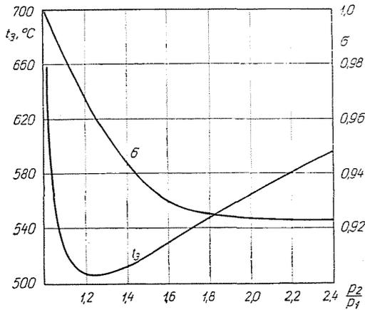
Fig. 3. Alteration of the  $t_3$  temperature of the test gas turbine and of the  $\sigma$  pressure loss factor in the function of the pressure ratio
