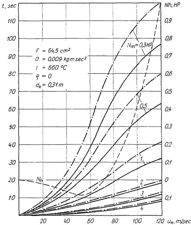
Fig. 11. "Warm" starting conditions of the test gas turbine ——— rated — — — — — measured (experimental) — — — — — useful power
