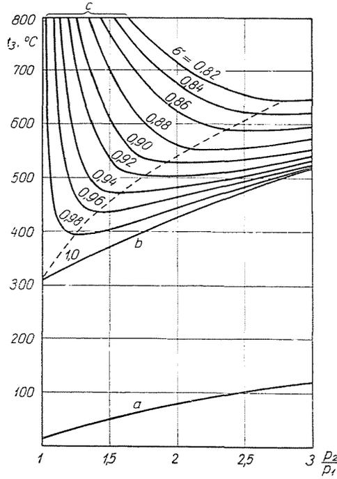
Fig. 2. Idling temperature of gas turbines in the function of the pressure ratio. a) ideal process, b) actual  $\eta_{adK} = \text{const}$ ;  $\eta_{adT} = \text{const}$ ; c) actual  $\eta_{adK} = \text{const}$ ;  $\eta_{adT} = \text{const}$ ;  $\sigma = \text{const}$
