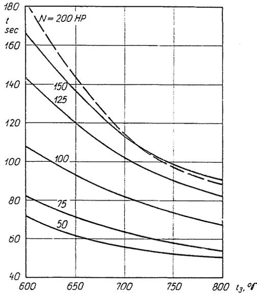
Fig. 13. The decrease of the starting time as a result of the  $t_3$  temperature-increase of gas turbines started by hand power
