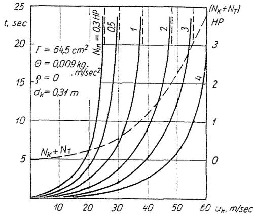
Fig. 10. Rated "cold" starting time of the test gas turbine
