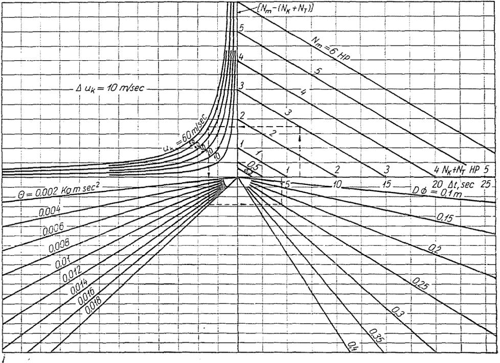
Fig. 7. For the determination of the speed-up time of the "cold" gas turbine
