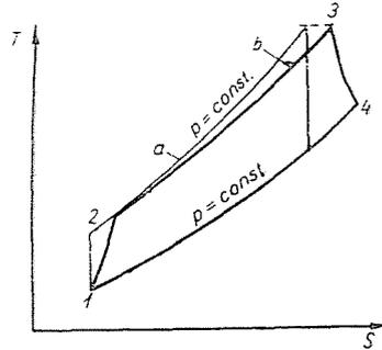
Fig. 1. TS diagram of the examined cycle. a) ideal cycle, b) actual (losing) cycle
