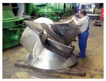
Fig. 10. Mixed flow pumps with prerotation unit in the factory.
