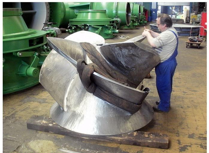
Fig. 10. Mixed flow pumps with prerotation unit in the factory.
