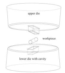
The schematic 3D view of the tools and the workpiece
