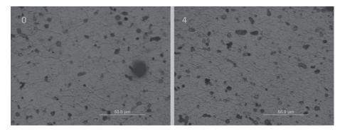
Fig. 8. Microstructure development during MF using optical microscopy; microstructure of the initial material and after the forth pass.
