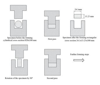
**Fig. 1.** The schematic 3D view of the tools and the workpiece and the principle of multiple forging using closed dies.
