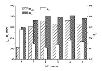
Fig. 4. Tensile strength  $(R_{p02})$ , yield stress  $(R_m)$  and maximum elongation (E\_) after multiple forging.
