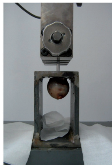
Fig. 11 Tensile test on a resected head of the femur
