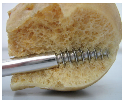
Fig. 2 Picture of a screw, fixing the neck of the femur, driven into the head of the femur (in section)
