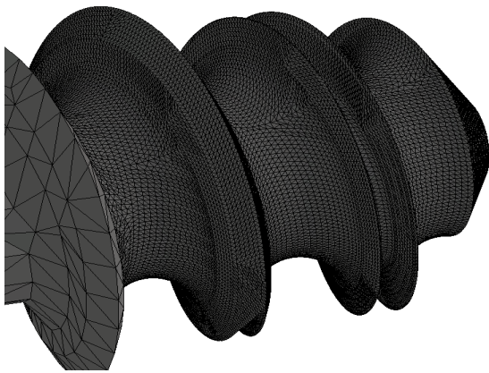
Fig. 5 A thickened finite element applied at the end of the screw (presented on a duplex screw)
