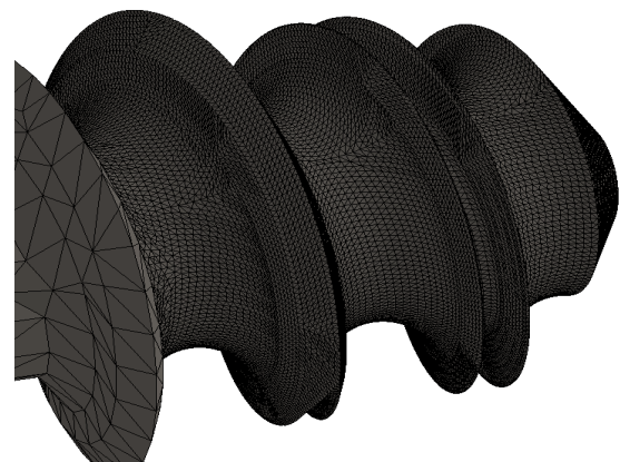
Fig. 5 A thickened finite element applied at the end of the screw (presented on a duplex screw)
