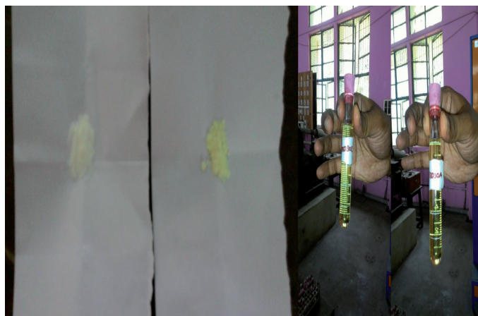
Fig. 2 Stability images of Alumina and Cerium Oxide nanoparticle test fuel
