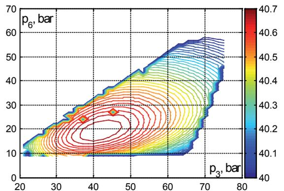
Fig. 2 2-dim search space of LANG-BBC 215 MW steam turbine
