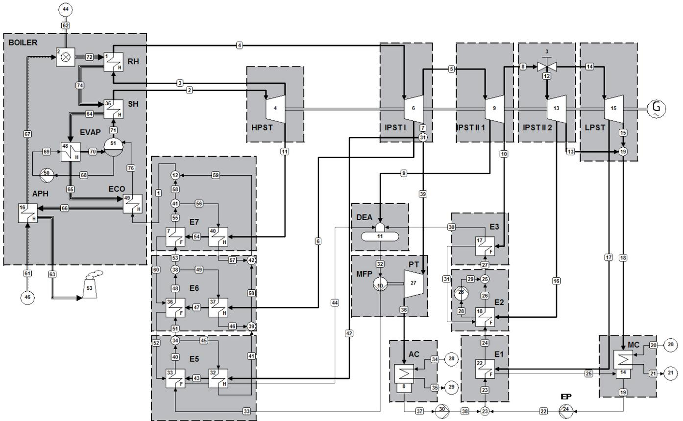
Fig. 1 Simplified scheme of the LANG-BBC 215 MW steam turbine cycle
