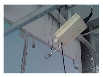
Fig. 3 Hot-wire anemometer probe
