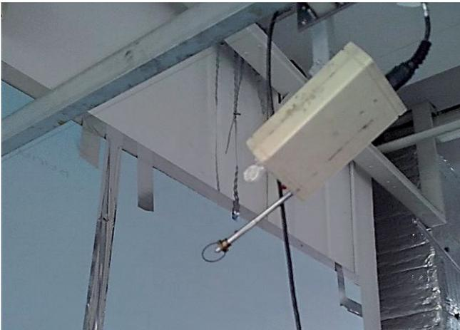
Fig. 3 Hot-wire anemometer probe
