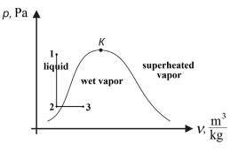
**Fig. 1** A diagram of the ideal process of fuel parameters changes in the standard fuel injection system: 2-1 is the process of increasing the fuel pressure with a pump, 1-2 is the process of dropping the fuel pressure when spraying through the injector, 2-3 is the process of heat supply from the inlet valve cap of a running engine to fuel, *K* is the critical point
