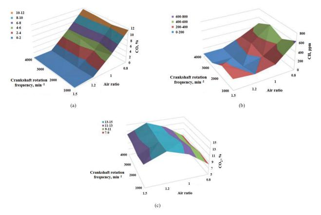
Fig. 7 The contents of (a) CO; (b) CH; and (c) CO<sub>2</sub> in the n-butanol combustion products.
