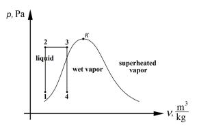
**Fig. 2** A diagram of the ideal process of fuel parameters changes in the multipoint superheated fuel injection system: 1-2 is the process of increasing the fuel pressure with a pump, 2-3 is the process of heat supply to fuel in the system of the superheated fuel injection, 3-4 is the process of dropping the fuel pressure when spraying with the system of superheated fuel injection, K is the critical point.
