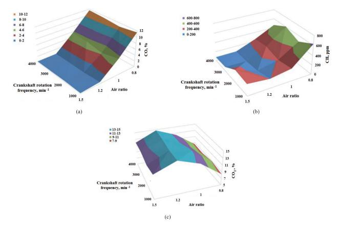
Fig. 4 The contents of (a) CO; (b) CH; and (c) CO, in the gasoline combustion products.
