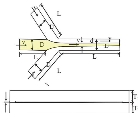
**Fig. 2** Scheme of the hydrodynamic flow focusing
