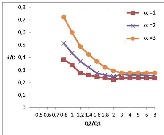
**Fig. 6** The effect of stream rate ratio ( $Q_1 / Q_2$ ) on glycerol nitration reaction with various length ratio ( $\alpha$ )
