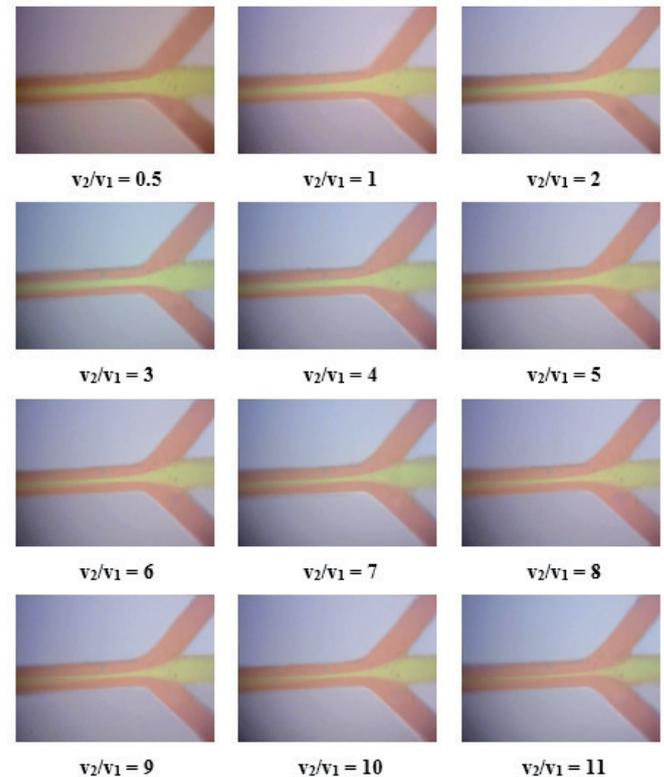
Fig. 4 The effect velocity ratio ( $v_1/v_2$ ) of glycerol nitration reaction
