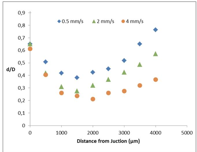
**Fig. 7** The velocity variations of core channel stream and sheath to focus width based on a range of the intersection.
