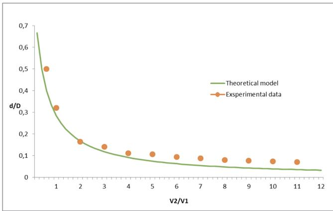
**Fig. 5** The effect of velocity ratio ( $v_1 / v_2$ ) on glycerol nitration reaction with the length ratio ( $a$ ) = 1.
