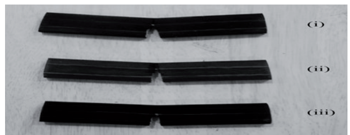
Fig. 2 Composite samples with no fibre discontinuity: (i) A1B1C1, (ii) A1B2C2, (iii) A1B3C3
