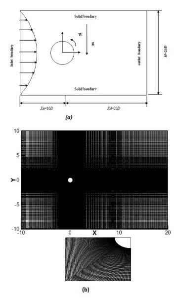
Fig. 1 (a) Schematic of the confined flow and heat transfer around a rotating circular cylinder (b) refining the mesh near the wall circular cylinder
