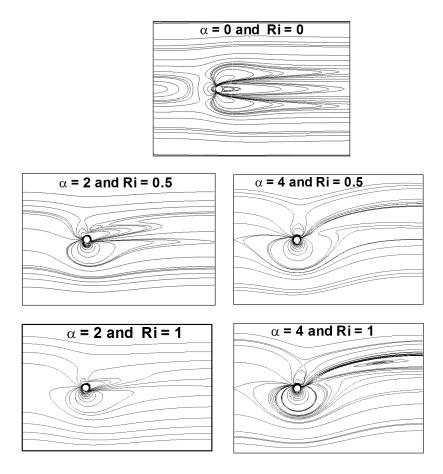
Fig. 7 Velocity field at Re = 40 for varying values of Ri and rotation rate
