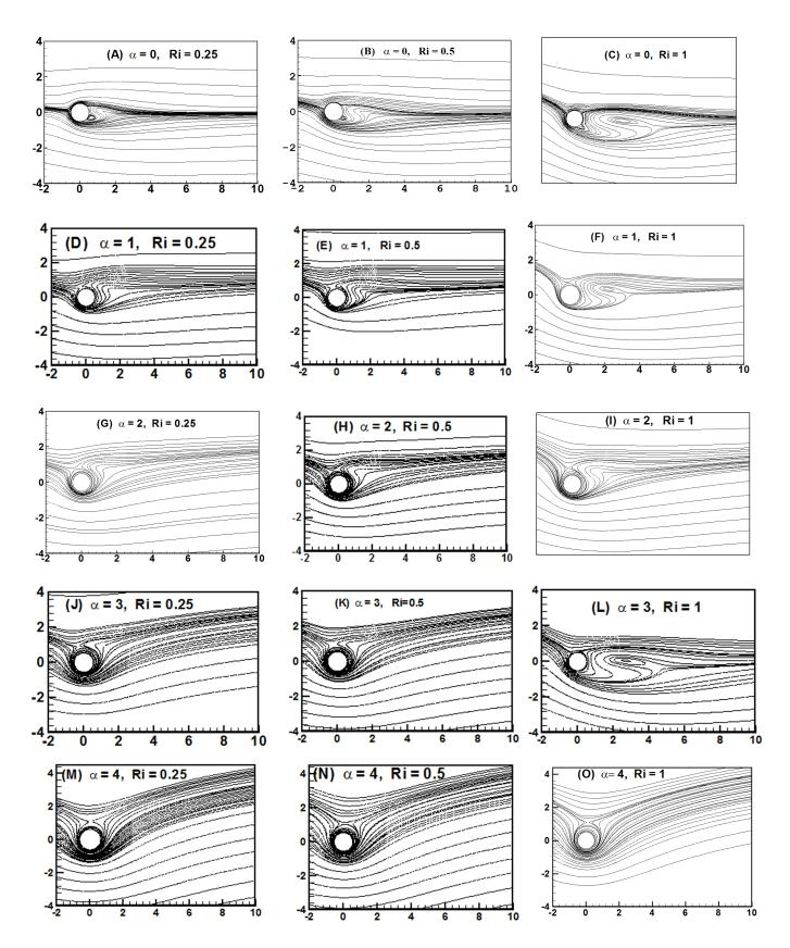
Fig. 3 The streamline profiles at Re = 20 for varying values of Richardson number and rotation rate
