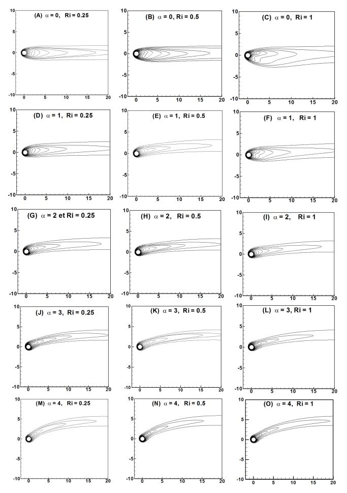
Fig. 6 Isotherm profiles at Re = 40 for varying values of Richardson number and rotation rate
