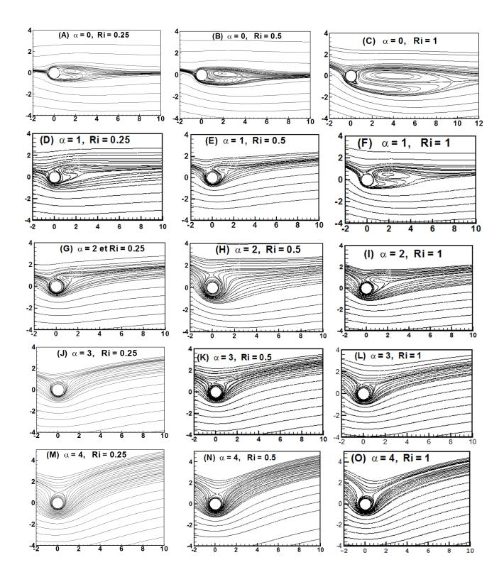
Fig. 4 The streamline profiles at Re=40 for varying values of Richardson number and rotation rate
