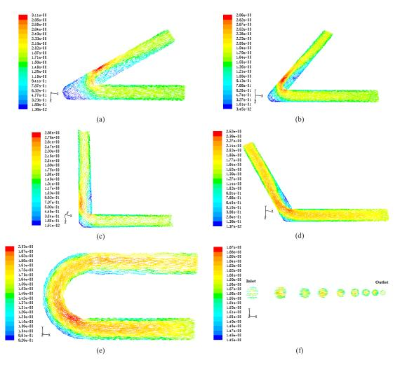
Fig. 7 Contour plot of velocity vector (m/s) of the bends (a) 30° (b) 60° (c)90° (d) 120° (e) U-bend and (f) straight pipe, SCMC solution Conc. (kg/m<sup>3</sup>): 0.8, Q<sub>1</sub>(m<sup>3</sup>/s): 20 x 10<sup>-5</sup>
