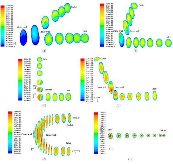
**Fig. 6** Contour plot of velocity magnitude (m/s) inside the different points of the bends (a) 30° (b) 60° (c) 90° (d) 120° (e) U-bend (f) straight pipe, SCMC solution Conc. (kg/m<sup>3</sup>): 0.8, Q<sub>1</sub>(m<sup>3</sup>/s): 20 x 10<sup>-5</sup>
