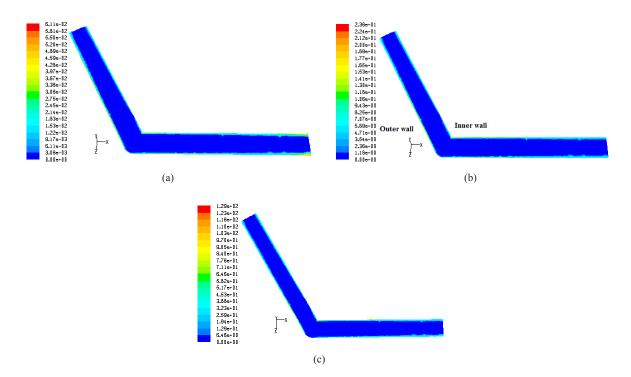
Fig. 19 Contour plot of wall shear stress (Pa) of the 120° bends for SCMC solution flow rate,  $Q_1(m^3/s)$ : 20 x 10<sup>-5</sup> and Conc. (kg/m<sup>3</sup>):, (a) water (b) 0.2 and (c) 0.8
