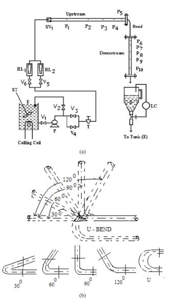
**Fig. 1** (a) Schematic diagram of the experimental set up for bends E - tank; P - pump; S - separator; P<sub>1</sub> - P<sub>10</sub> - manometer toppings; LC - level controller; RL<sub>1</sub> - RL<sub>2</sub> - rota meters; ST - stirrer; SV<sub>1</sub> - solenoid valve; V<sub>1</sub> - V<sub>6</sub> - valves. (b) Types of bends.
