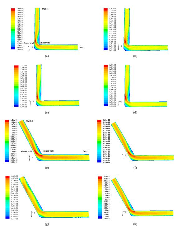
Fig. 15 Contour plot of velocity magnitude (m/s)(a)- (b) for 90° bends and (e) -(f) for 120° bends for SCMC solution Conc. (kg/m<sup>3</sup>): 0.8 and (c) - (d) for 90° bends and (g) -(h) for 120° bends for water at low and high flow rate  $Q_i(m^3/s)$ : 14.12 x 10<sup>-5</sup> and 20 x 10<sup>-5</sup>
