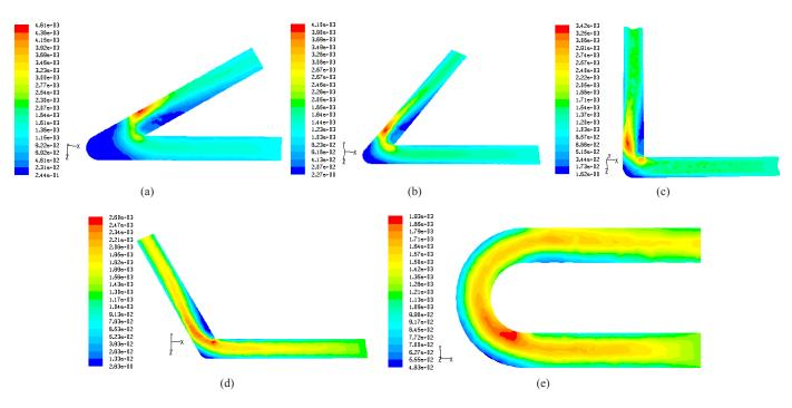
Fig. 10 Contours of dynamic pressure (Pa) of the bends (a) 30° (b) 60° (c) 90° (d) 120° (e) U-bend, SCMC solution Conc. (kg/m<sup>3</sup>): 0.8, Q<sub>1</sub>(m<sup>3</sup>/s): 20 x 10<sup>-5</sup>
