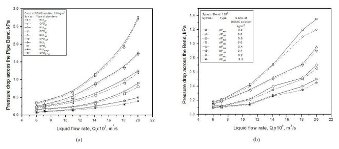
Fig. 22 (a) variation of pressure drop across the bends with liquid flow rate (b) comparison plot of pressure drop across the bends versus liquid flow rate at different SCMC solution concentration (kg/m<sup>3</sup>): 0.2 - 0.8
