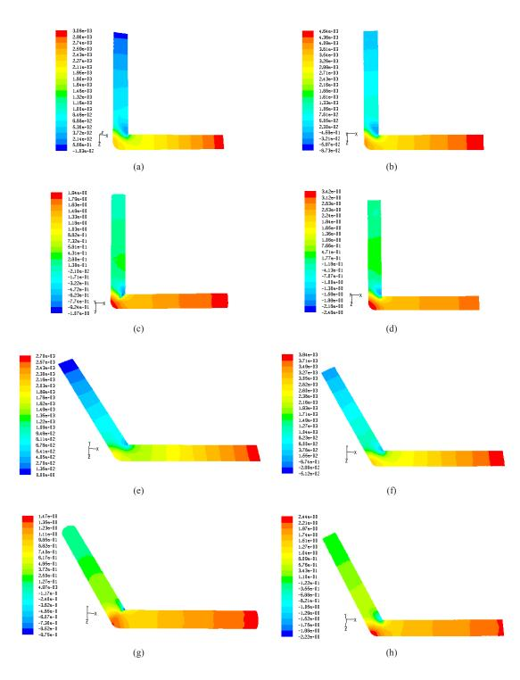
Fig. 14 Contour plot of static pressure (Pa) (a) - (b) for 90° bends and (e) -(f) for 120° bends for SCMC solution Conc. (kg/m<sup>3</sup>): 0.8 and (c) - (d) for 90° bends and (g) -(h) for 120° bends for water at low and high flow rate  $Q_1(m^3/s)$ : 14.12 x 10<sup>-5</sup> and 20 x 10<sup>-5</sup>
