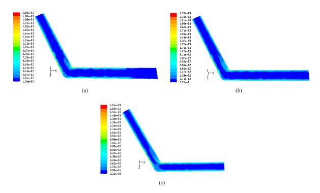
Fig. 20 Contour plot of wall strain rate (1/s) of the 120° bends for SCMC solution flow rate,  $Q_1(m^3/s)$ : 20 x 10<sup>-5</sup> and Conc. (kg/m<sup>3</sup>):, (a) water (b) 0.2 and (c) 0.8
