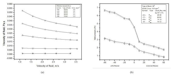
Fig. 21 (a) Variation of viscosity with fluid velocity for SCMC solution and water, (b) comparison plot of experimental and CFD for 30° bend
