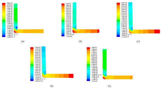
Fig. 17 Contour plot of static pressure (Pa) inside the different points of the90° bends for SCMC solution flow rate,  $Q_1(m^3/s)$ : 20 x 10<sup>-5</sup> and Conc. (kg/m<sup>3</sup>): (a) 0.2 (b) 0.4 (c) 0.6 (d) 0.8 (e) water.
