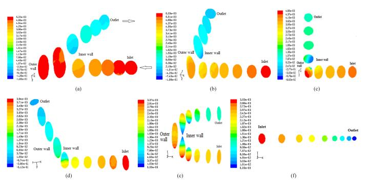
Fig. 4 Contour plot of static pressure (Pa) inside the different points of the bends (a) 30° (b) 60° (c) 90° (d) 120° (e) U-bend (f) straight pipe, SCMC solution Conc. (kg/m<sup>3</sup>): 0.8, Q(m<sup>3</sup>/s): 20 x 10<sup>-5</sup>
