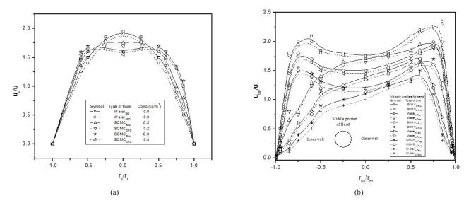
Fig. 23 Velocity profiles for water and SCMC solution flow through (a) straight pipe and (b) bends
