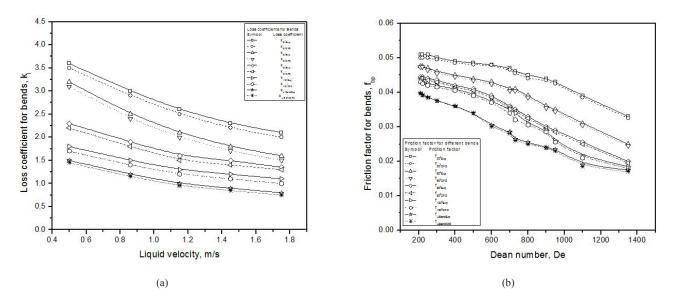
Fig. 24 Comparison plot of experimental and CFD simulated data for (a) loss coefficients of different types of bends with 0.8 kg / m<sup>3</sup> SCMC solution (b) friction factor vs. Dean Number
