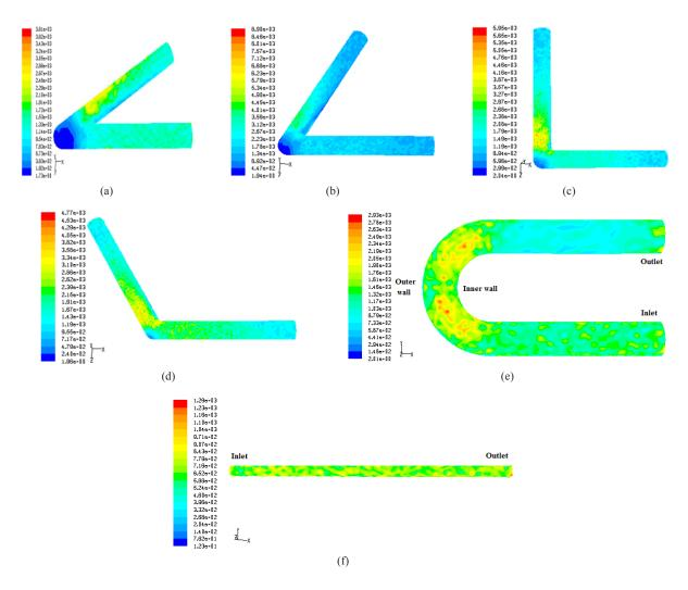
Fig. 13 Contour plot of shear strain rate (1/s) of the bends (a) 30° (b) 60° (c) 90° (d) 120° (e) U-bend (f) straight pipe, SCMC solution Conc. (kg/m<sup>3</sup>): 0.8, Q<sub>1</sub>(m<sup>3</sup>/s): 45 x 10<sup>-5</sup>
