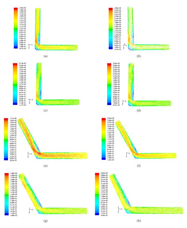
Fig. 16 Contour plot of velocity vector (m/s) (a) - (b) for 90° bends and (e) -(f) for 120° bends for SCMC solution Conc. (kg/m<sup>3</sup>): 0.8 and (c) - (d) for 90° bends and (g) -(h) for 120° bends for water at low and high flow rate  $Q_1(m^3/s)$ : 14.12 x 10-5 and 20 x 10-5
