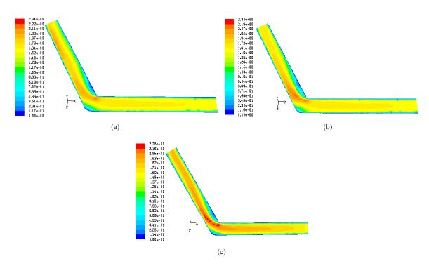
Fig. 18 Contour plot of velocity magnitude (m/s) of the 120° bends for SCMC solution flow rate, Q<sub>1</sub>(m<sup>3</sup>/s): 20x 10<sup>-5</sup> and Conc. (kg/m<sup>3</sup>): (a) water (b) 0.2 and (c) 0.8
