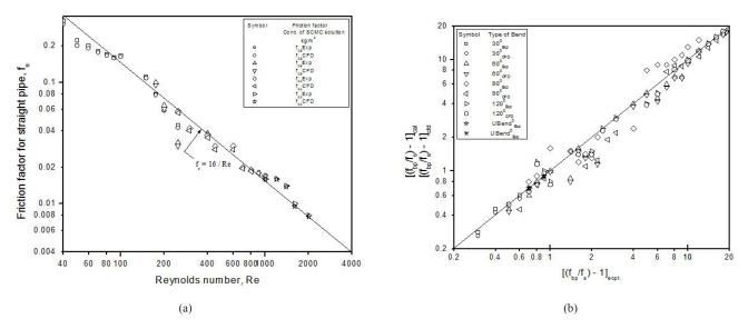
**Fig. 25** (a) Plot of  $f_s$  vs. Re for straight pipe (b) Plot of  $[(f_{bn}/f_s) - 1]_{cal}$  vs.  $[(f_{bn}/f_s) - 1]_{ext}$  for all types of bends in horizontal plane.
