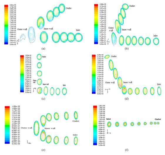
Fig. 8 Dean vortices inside the different points of the bends (a) 30° (b) 60° (c) 90° (d)120°
