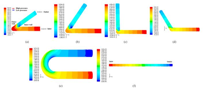
**Fig. 3** Contour plot of static pressure (Pa) of the bends (a) 30° (b) 60° (c) 90° (d) 120° (e) U-bend (f)straight pipe, SCMC solution Conc. (kg/m<sup>3</sup>): 0.8, Q<sub>1</sub>(m<sup>3</sup>/s): 20 x 10<sup>-5</sup>
