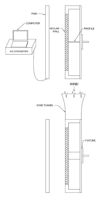
Fig. 2 Measurement setup from two perspectives
