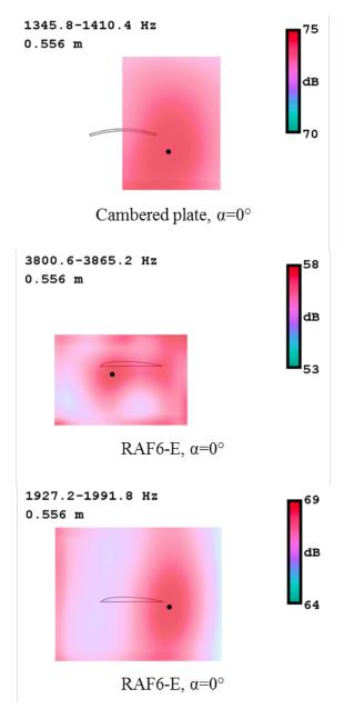
Fig. 6 Beamforming source maps: profile/blunt TE vortex shedding (top), blunt TE vortex shedding (middle), profile vortex shedding (bottom). The SSL maxima are marked with black dots.
