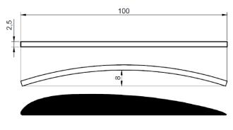
Fig. 1 The cross-sections of the flat plate (top), the cambered plate (middle) and the RAF6-E [6] (bottom)
