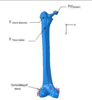
Fig. 4 Representation of the boundary conditions imposed on the analyzed structure
