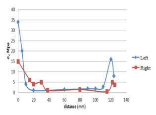
Fig. 15 Von-misses stress ( $\sigma e$ ) in climb stairs activity of the left and right side of PMMA cement.
