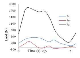
**Fig. 1** Decomposition of a normal operating cycle Corresponding to the efforts applied to the femoral head
