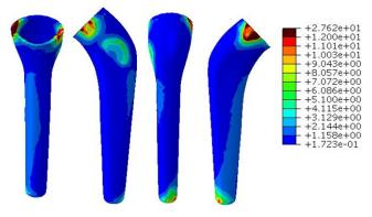
Fig. 7 Von-mise stress induced in the cement during a normal walking cycle at the max point (t = 0.19s).
