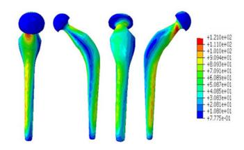
Fig. 5 Constraint Von Mises induced in the implant during a cycle of normal walking to the max point at t = 0.19s
