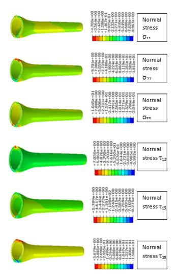
Fig. 8 Normal and tangential stresses induced in PMMA cement when climbing stairs at max point T = 0.3s
