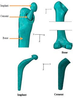
Fig. 3 The conception of the model CMK 3 with Software ABAQUS (mesh boundary)
