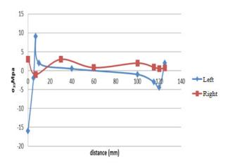
Fig. 11 Stress  $\sigma$ 33 in climb stairs activity of the left and right side of PMMA cement
