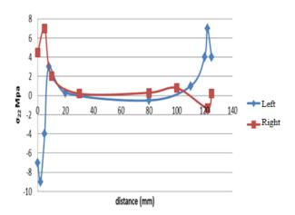
Fig. 10 Stress  $\sigma$ 22 in climb stairs activity of the left and right side of PMMA cement
