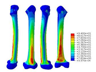
Fig. 6 Von Mises Stress induced in the bone during a cycle of normal walking at max point t = 0.19s.
