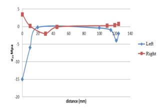
Fig. 14 Stress  $\tau$  23 in stair climbing activity of the left and right side of PMMA cement.
