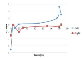
Fig. 13 Stress  $\tau$  13 in climb stairs activity of the left and right side of PMMA cement
