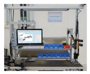
Fig. 12 Manual assembly workstation equipped with a touchscreen (Schuh et al., 2015)
