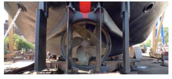
Fig. 4 Screw, tunnel, nozzle and rudder arrangement fitten on the HERSO 1
