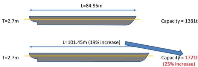
Fig. 5 Retrofit option No.1: Ship hull lengthening
