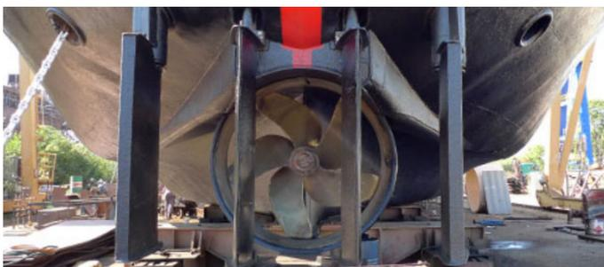
Fig. 4 Screw, tunnel, nozzle and rudder arrangement fitted on the HERSO 1
