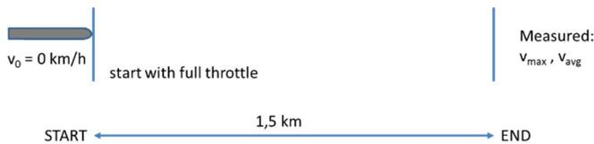
Fig. 10 Illustration of speed change measurement test
