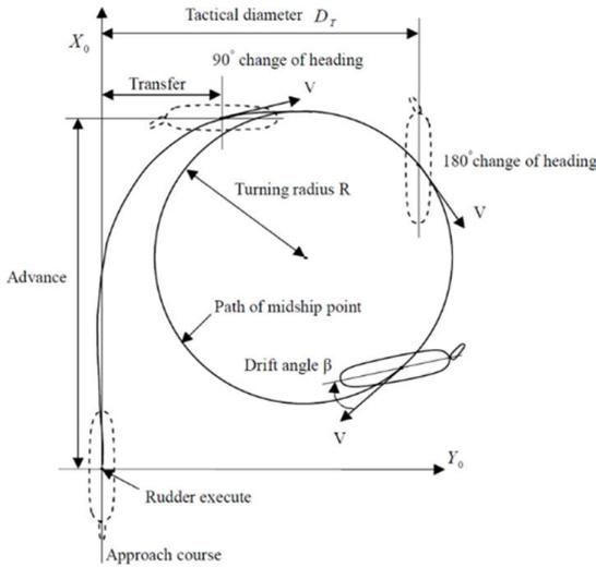
Fig. 8 Parameters of a turning circle test
