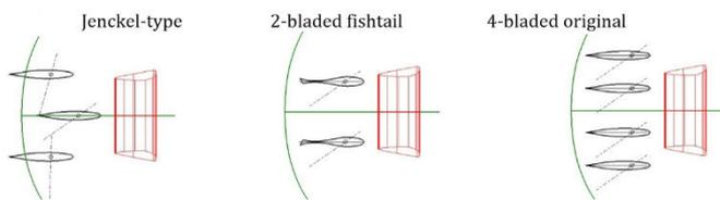
Fig. 6 Retrofit option No.2: Rudder configuration changes
