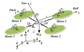
Fig. 2 The structure of quadrotor and relative coordinate systems.
