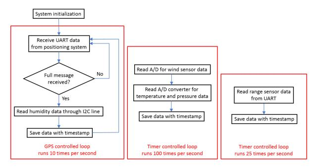
Fig. 5 Basic flowchart of DAQ controller firmware
