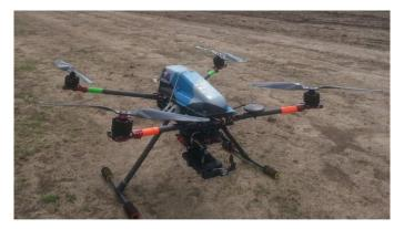
Fig. 2 Dropbear quadcopter from Australian Droid and Robot (ADR)
