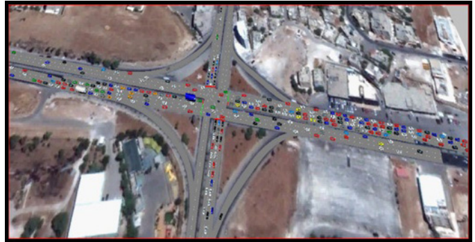
Fig. 3 VISSIM Simulation for the Existing Conventional Intersection
