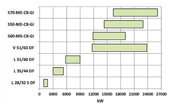
Fig. 1 The distribution of "MAN Diesel & Turbo SE" dual-fuel engines power range
