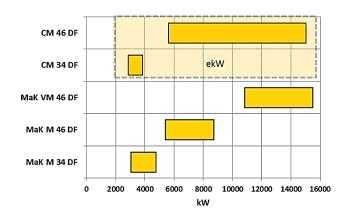
Fig. 2 The distribution of "Caterpillar Inc." and "MaK" dual-fuel engines power range
