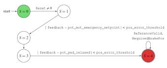
Fig. 6 High Level Control Logic: State machine
