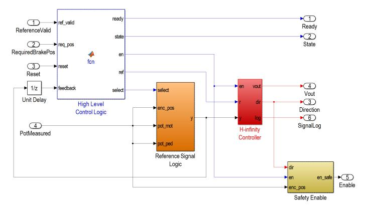
Fig. 5 Block diagram of the controller
