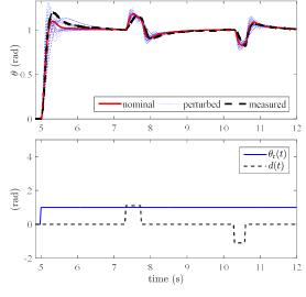
Fig. 10 Step response in closed loop
