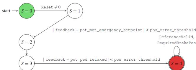
Fig. 6 High Level Control Logic: State machine
