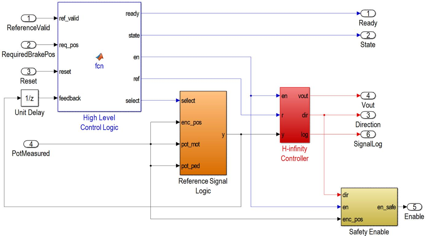
Fig. 5 Block diagram of the controller
