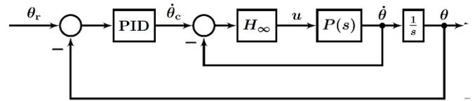
Fig. 2 Cascade control loop
