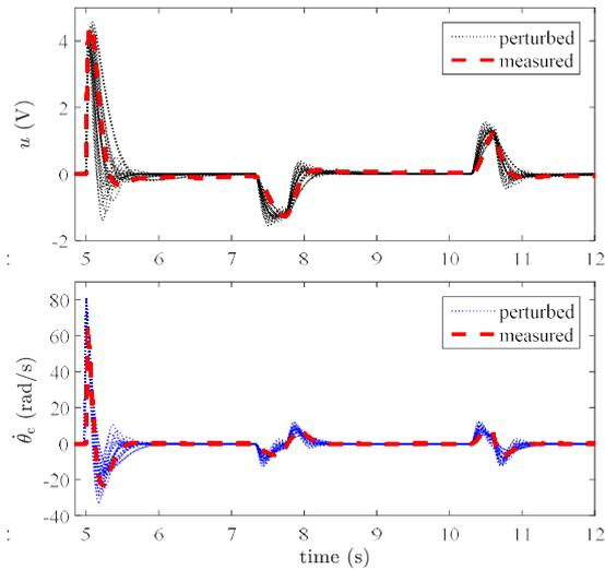
**Fig. 11** H-infinity (top) and PID (bottom) control signals of prototype system
