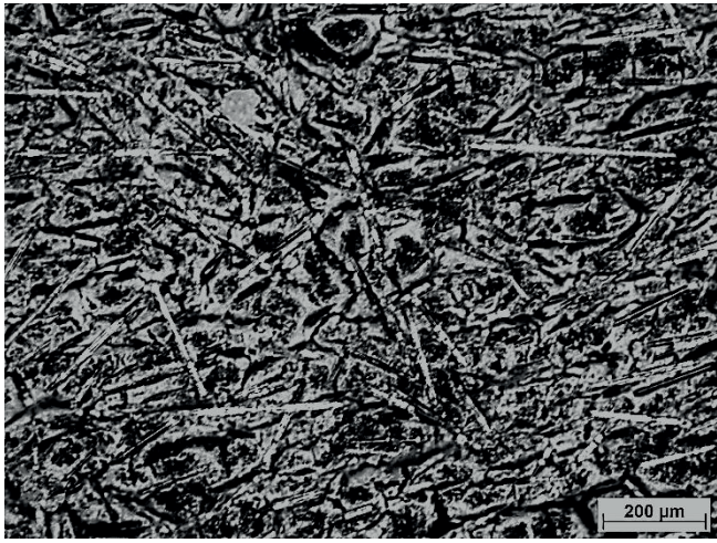
Fig. 6 Surface structure of the tested composites with 30 % of glass fibers content after 1000 hours exposition in UV box
