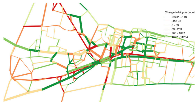
Fig. 5 Change in bicycle count for business-as-usual scenario with respect to BSH-b policy scenario (green and red colors represent a decrease and increase in bicycle traffic respectively). Thicker lines represent higher capacities of links (e.g. arterials).
