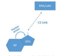
Fig. 2 Elements of an UAS/RPAS
