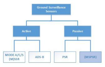
Fig. 5 Surveillance sensors classification
