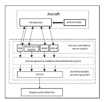
Fig. 4 Elements of the surveillance chain
