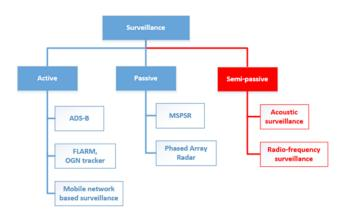
Fig. 6 Extended surveillance sensors classification
