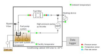
Fig. 2 Proposed new diesel cold start measurement system
