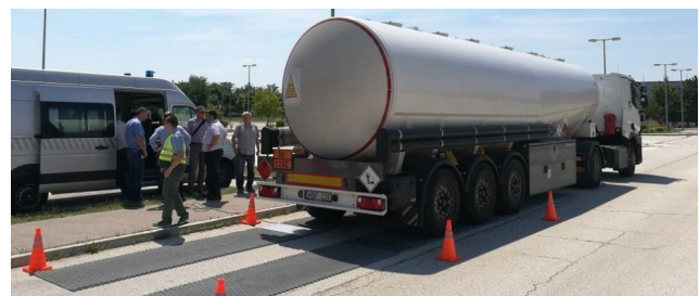
Fig. 2 Axle load measurement of special reference vehicle (Ronay-Tobel et al., 2019)
