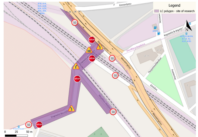
Fig. 2 The RRLC - site of research, the pre-defined polygon and the vertical signing elements of the road network
