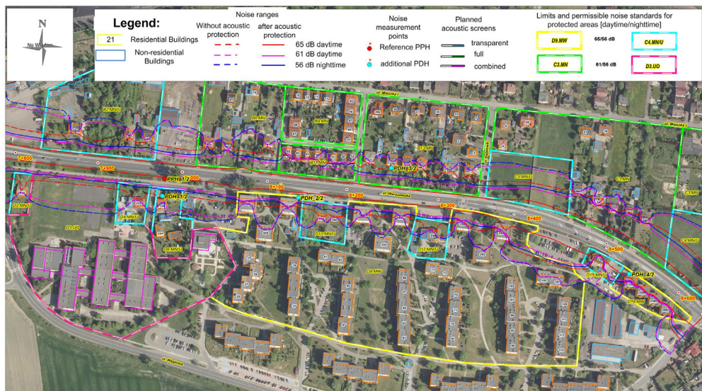
Fig. 6 Map of noise impact ranges at the height of 4 m above ground level without and after the application of noise protection in the form of a quiet pavement
