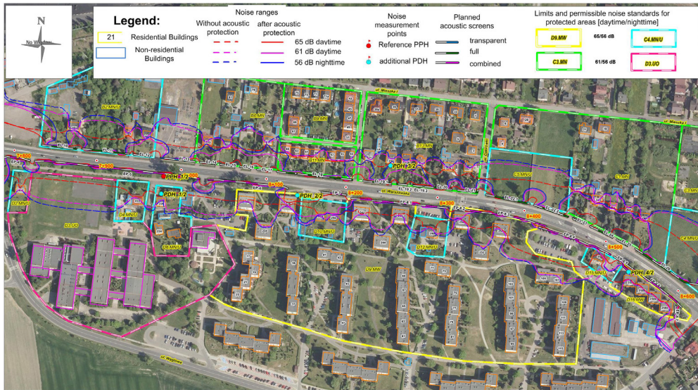
Fig. 5 Map of noise impact ranges at the height of 4 m above ground level before and after the application of acoustic protection in the form of screens
