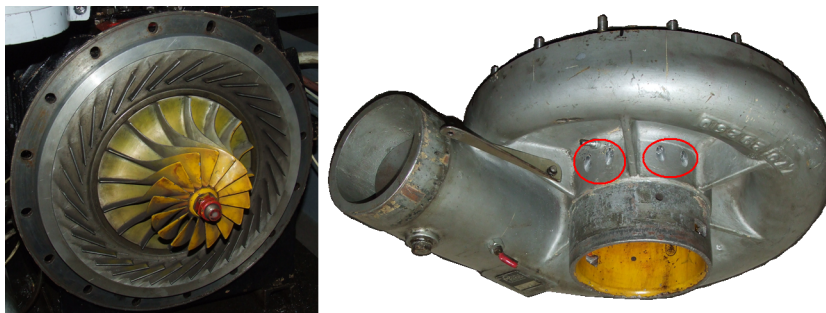
Fig. 1. The impeller of the GANZ compressor with scroll removed (left) and the modified scroll with shroud bleed orifices (right)
