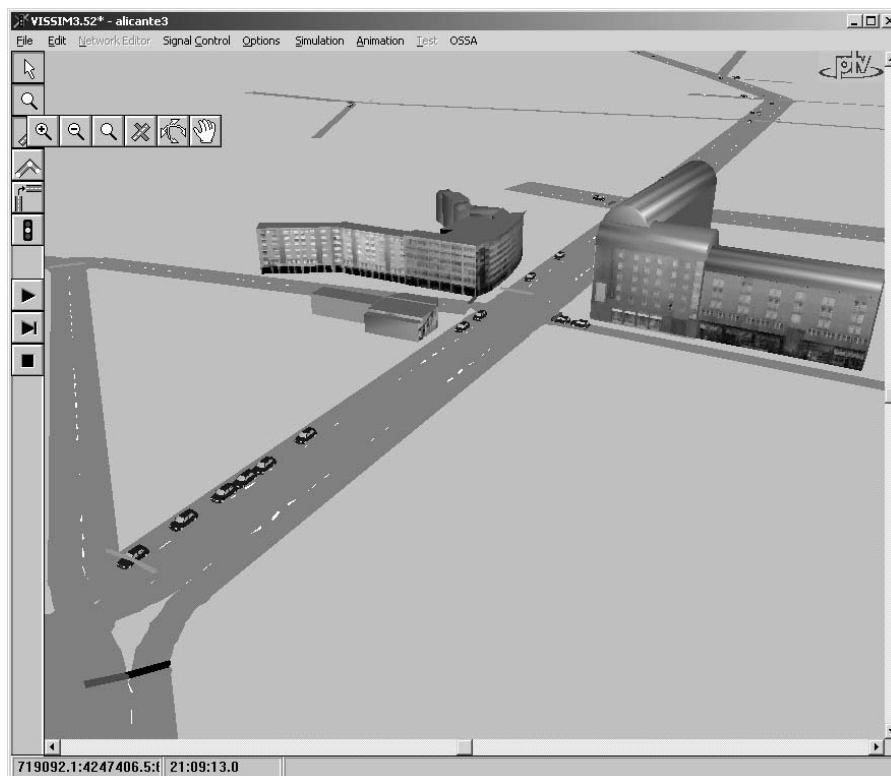
Fig. 8. The visualizer module shows the actual state of the traffic during the simulation
