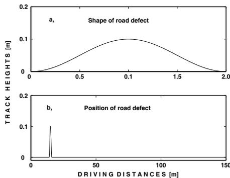
*Fig. 2.* The applied road defect
