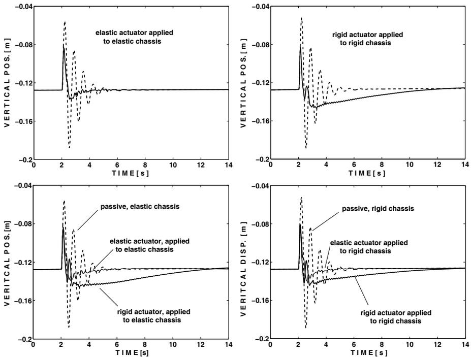
Fig. 3. Straight motion. The vibration of the chassis at the right-hand-side front suspension
