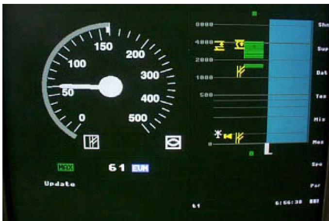
Fig. 5. MMI – simulation of the ETCS onboard equipment
