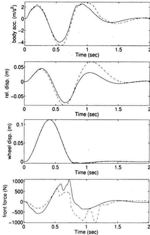
Fig. 5. Time responses of the controlled system using an LPV and a  $\mathcal{H}_\infty$  control
