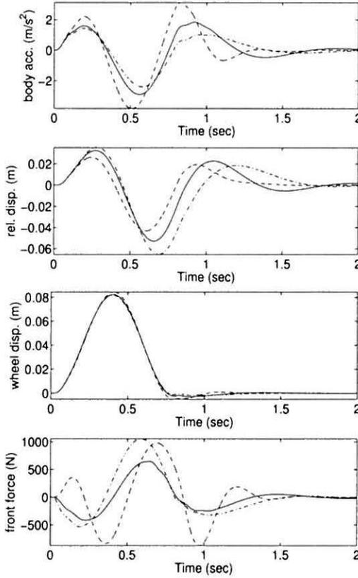
Fig. 4. Time responses of the controlled system using LPV controllers
