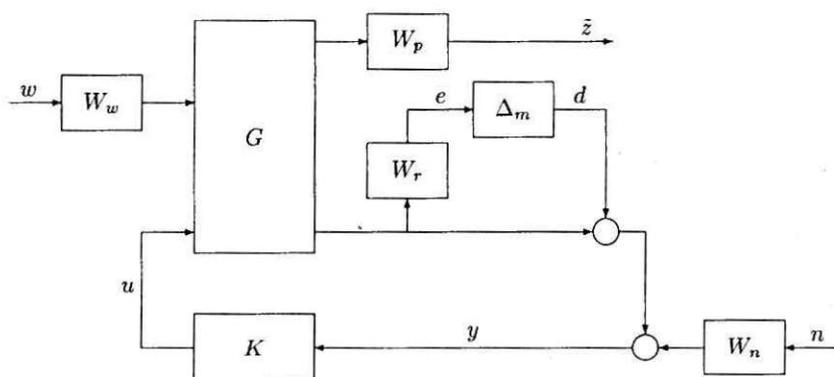
Fig. 2. The closed-loop interconnection structure
