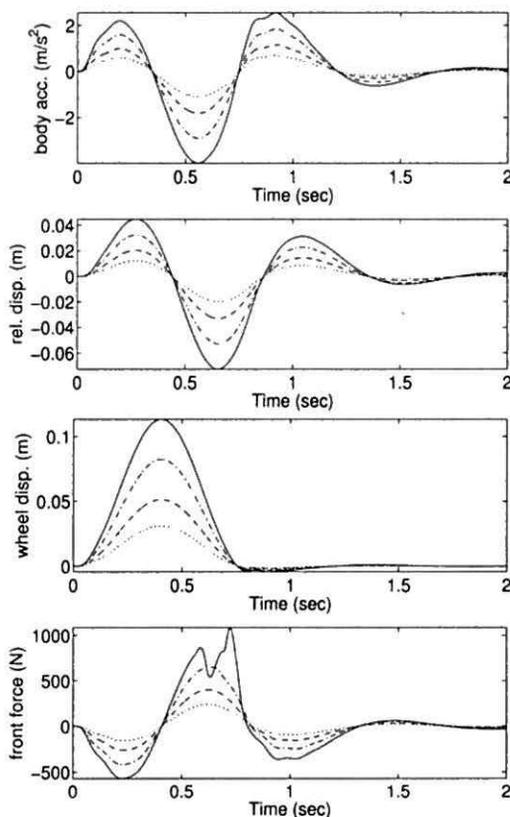
Fig. 3. Time responses of the nonlinear controlled system using LPV controllers for different bumps
